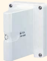
YW-4500 UHF Wireless Antenna • UHF wireless dipole indoor antenna • Wall mounted • Power supplied by tuner unit (WT-5800/WT-5805/WT-4820) through coaxial cable • Built-in RF signal booster • Attenuation switch helps minimize noise and any interference.
